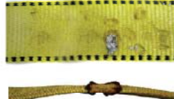
Sling Weld Splatters and Charring/Melting
