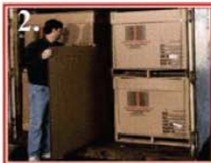
Step 2: Protect the bag from sharp objects
