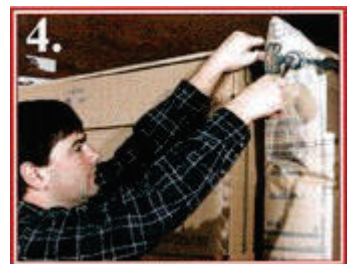
Step 4: Inflate the bag till the cargo is properly secured
