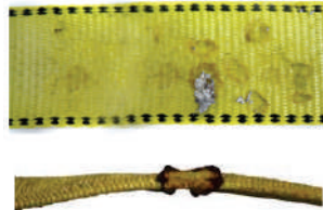
Sling Weld Splatters and Charring/Melting
